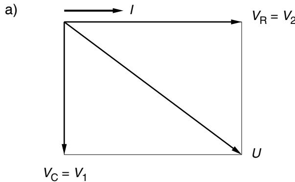
$$\text{b) } X_C = \frac{V_1}{I} = 115 \Omega$$
